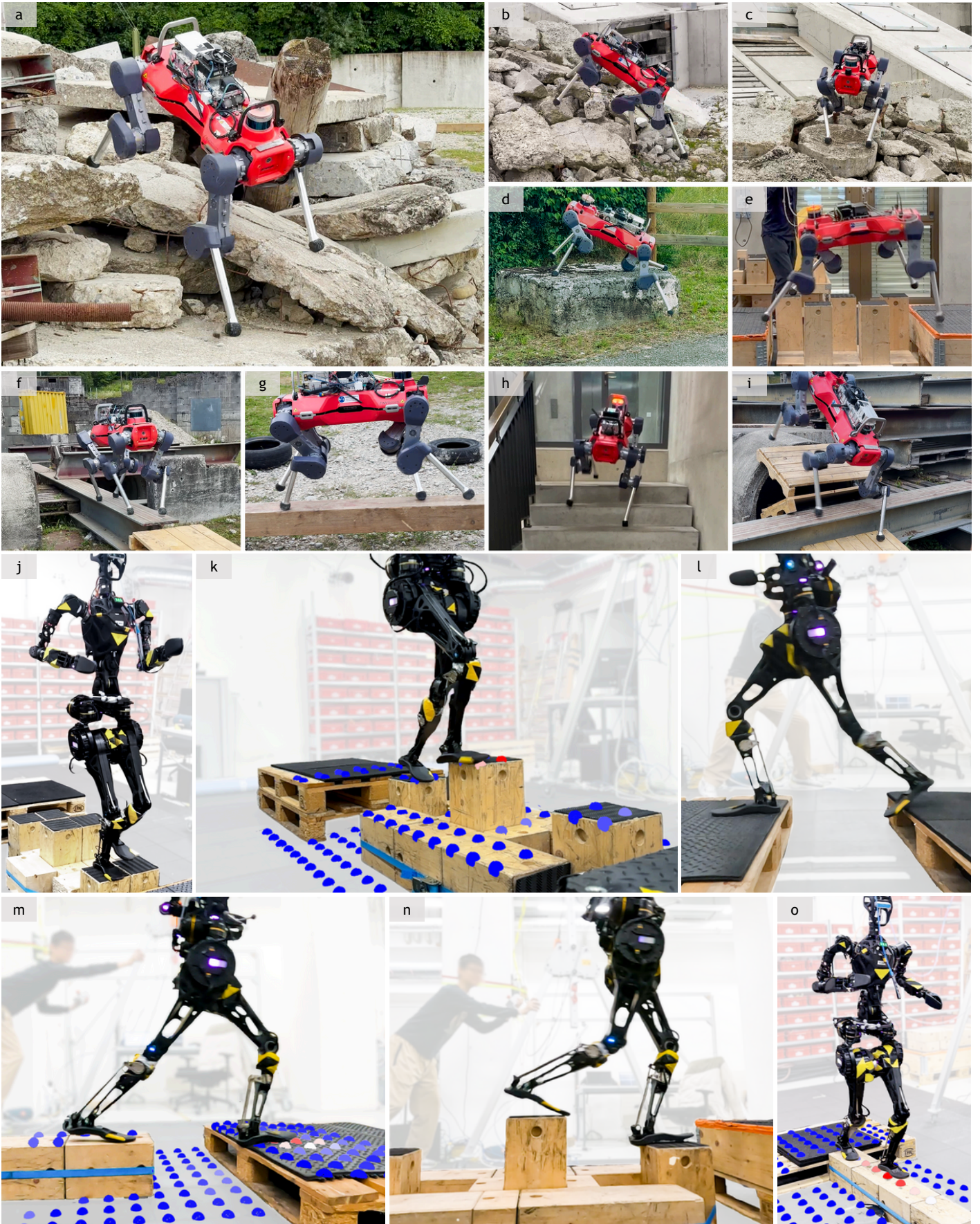
Fig. 1. Learning interpretable, generalizable, agile, and robust legged locomotion on diverse terrains. Our end-to-end controllers enabled ANYmal-D (a - i) and GR-1 (j - o) to dynamically traverse diverse challenging terrains. Highly interpretable point-wise map encodings are graphically visualized in k, m, and o, where colors more intense in red represent higher attention weights, indicating the next foothold.
