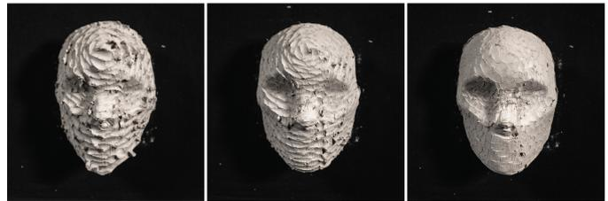
Fig. 23. The abstract face model sculpted with different tools and in different toolpath densities: left – 250 toolpaths, round tool; middle – 400 toolpaths, round tool; right – 400 toolpaths, flat tool.
