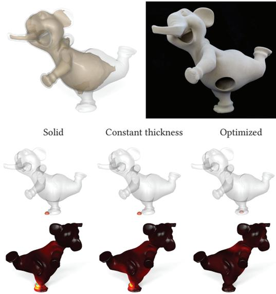
Fig. 7. Our *Elephant* is optimized to balance under self-weight (top). For the solid model (bottom left), the projected center of mass lies outside the support polygon. The visualization of the failure potential (bottom) shows that the model would break if fixed to the ground (blue region). The constant thickness model (bottom center), while structurally sound, would topple over. Our optimized model (bottom right) is sound *and* stands stably (see also image of printed model).
