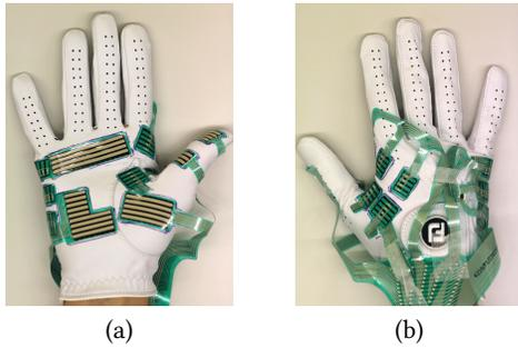
**Figure 1: Pressure sensitive glove with Tekscan Grip System. Although this works well for human-human interaction, the limited sensing area makes it unsuited for robot hands with varying morphologies.**
