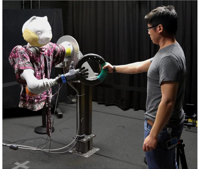
Fig. 1. The robotic character can perform both human-to-robot and robot-to-human handovers.
