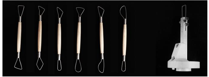
**Fig. 3.** Left: different manual loop tools used by professional sculptors; Right: our customized loop tool that can be attached to a UR5 as the robot end effector.
